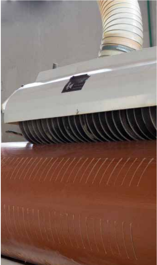
The method of producing perforations in the PVC pipes
