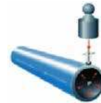
Point load test according to dr. Hessel
