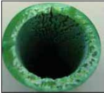
Picture no. 53: The appearance of degraded PP-R and PP-RCT tubes due to the action of negative copper ions
