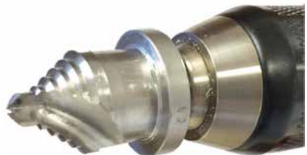
Picture no. 28: Auger for drilling holes in the pipes
