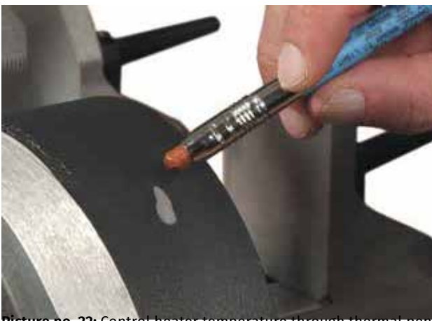
Picture no. 22: Control heater temperature through thermal pen
