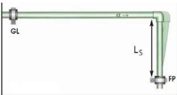
Picture no. 60: Display of the correct acceptance of longitudinal dilatations by changing the direction, where GL is a plain bearing (support), and FP fixed bearing (fixed support), while L_s is required length of change direction.
