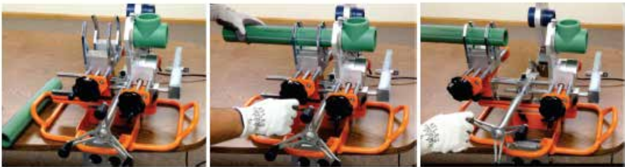
Picture no. 37: Pipe and fitting alignment procedure
