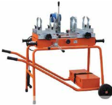
Picture no. 36: Welding machine with stand
