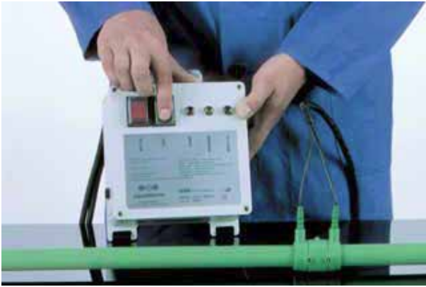
Picture no. 34: Indicates the power of the EF device connected to the EF connector in the correct way
