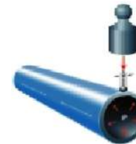
Point load test according to dr. Hassel
